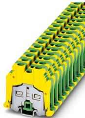
Ground terminal, When aligned with a feed-through terminal block of the same shape, a partition plate must be used for insulation voltages > 250 V, number of connections: 2, connection method: Screw connection, 1 level, cross section: 0.5 mm<sup>2</sup> - 10 mm<sup>2</sup>, mounting: PE foot with mounting screw, M4, mounting type: NS 15, color: green-yellow
