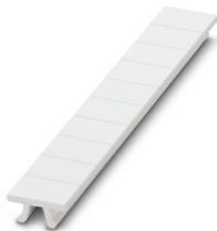
Zack marker strip, Strip, white, unlabeled, can be labeled with: CMS-P1-PLOTTER, PLOTMARK, mounting type: snapped, for terminal block width: 8.2 mm, lettering field size: 10.5 x 8.15 mm, Number of individual labels: 10
