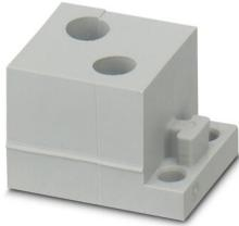
Cable sleeve, small, no. of conductors: 2, type: Round cable, slotted, external cable diameter: 2x 6.4 mm ... 6.7 mm, material: SEBS (halogen-free), color: gray, length: 29.5 mm, width: 19.5 mm, height: 17 mm
