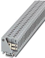
Mini feed-through terminal block, nom. voltage: 400 V, nominal current: 16 A, 1 level, connection method: Spade connection, cross section: 0.5 mm<sup>2</sup> - 1 mm<sup>2</sup>, mounting: NS 15, color: gray
