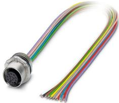
Device connector front mounting, Universal, 12-position, Socket, straight, M12-Standard, coding: A, on free cable end, Front mounting, Individual wires, cable length: 0.5 m, 0.14 mm<sup>2</sup>, TPE litz wire, Alternative product in accordance with RoHS II without Exemption 6c (Pb <0.1%) item no.: 1238715
