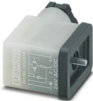
Valve connectors, Universal, 3-position, Valve connector B (10 mm), Screw connection, cable gland M16, external cable diameter 6 mm ... 8 mm
