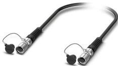
M17 series with preassembled FO plug assembly: 4-pos. plug-plug, multimode fiberglass G62.5/125  $\mu\text{m}$  OM1, with screw connection, length of FO cable: 120 m, IP67 degree of protection after being inserted, fixed installation in cable ducts, underground cable ducts, and cable protection pipes for indoor/outdoor use
