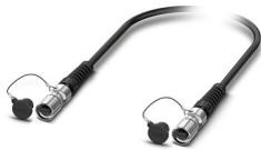
M17 series with preassembled FO plug assembly: 4-pos. plug-plug, multimode fiberglass G62.5/125  $\mu\text{m}$  OM1, with screw connection, length of FO cable: 40 m, IP67 degree of protection after being inserted, fixed installation in cable ducts, underground cable ducts, and cable protection pipes for indoor/outdoor use
