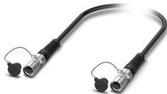
M17 series with preassembled FO plug assembly: 4-pos. plug-plug, multimode fiberglass G62.5/125  $\mu\text{m}$  OM1, with screw connection, length of FO cable: 50 m, IP67 degree of protection after being inserted, fixed installation in cable ducts, underground cable ducts, and cable protection pipes for indoor/outdoor use
