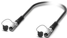
M17 series with preassembled FO plug assembly: 4-pos. plug-plug, multimode fiberglass G62.5/125  $\mu\text{m}$  OM1, with screw connection, length of FO cable: 140 m, IP67 degree of protection after being inserted, fixed installation in cable ducts, underground cable ducts, and cable protection pipes for indoor/outdoor use
