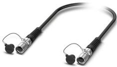
M17 series with preassembled FO plug assembly: 4-pos. plug-plug, multimode fiberglass G62.5/125  $\mu\text{m}$  OM1, with screw connection, length of FO cable: 20 m, IP67 degree of protection after being inserted, fixed installation in cable ducts, underground cable ducts, and cable protection pipes for indoor/outdoor use
