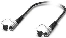
M17 series with preassembled FO plug assembly: 4-pos. plug-plug, multimode fiberglass G62.5/125  $\mu\text{m}$  OM1, with screw connection, length of FO cable: 110 m, IP67 degree of protection after being inserted, fixed installation in cable ducts, underground cable ducts, and cable protection pipes for indoor/outdoor use
