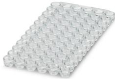
Guide element/front plate for the easy and secure connection of HC-DD series high-position connectors. Snap onto the contact insert. During connection, the pin contact is guided into place first, preventing contact with the socket contact.
