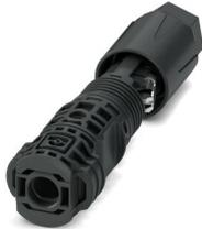
Photovoltaic connector, Range of articles: SUNCLIX, Connector, housing material: PPE, color: black, number of positions: 1, min. conductor cross section: 6 mm<sup>2</sup>, max. conductor cross section: 16 mm<sup>2</sup>, rated voltage: 1500 V DC, rated current: 60 A, Connection method: Spring-cage, Contact connection type: Pin, min. cable diameter: 5.5 mm, max. cable diameter: 10 mm
