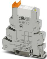
PLC-INTERFACE for protection against interference currents/voltages on the control side. Consisting of PLC-BSC-230UC/21HC/SO46 basic terminal block with screw connection and plug-in miniature relay with power contact up to 10 A, 1 changeover contact, 230 V AC input voltage
