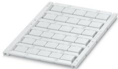
Marker for terminal blocks, can be ordered: by sheet, white, labeled according to customer specifications, mounting type: snap into tall marker groove, for terminal block width: 12 mm, lettering field size: 10.8 x 9.6 mm, Number of individual labels: 30
