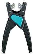
Stripping pliers, for halogen-free sensor/actuator cables (SAC cables), with PUR and PVC insulation, from Ø of 4.4 to 7 mm, any stripping length
