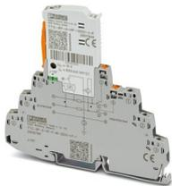
Surge protection, consisting of protective plug and base element, with integrated status indicator and knife disconnection for three signal wires with common reference potential. For HF applications and telecommunications interfaces without supply voltage. Indirect grounding via gas discharge tube, Ex e approval for zone 2.
