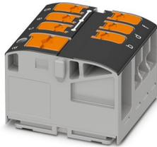
Distribution block, nom. voltage: 450 V, nominal current: 24 A, number of connections: 7, number of positions: 1, connection method: Push-in connection, Load contact, Rated cross section: 2.5 mm<sup>2</sup>, cross section: 0.14 mm<sup>2</sup> - 4 mm<sup>2</sup>, Line contact, Rated cross section: 6 mm<sup>2</sup>, cross section: 0.5 mm<sup>2</sup> - 10 mm<sup>2</sup>, mounting type: adhesive, color: black
