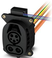
CHARX connect universal, Vehicle charging inlet, for charging with alternating current (AC) and with direct current (DC), CCS type 1, IEC 62196-2, IEC 62196-3, 250 A / 1000 V (DC), 80 A / 250 V (AC), Single wires, length: 2 m, locking actuator: 12 V, 4-pos., Front and rear mounting, M6, housing: black, A protective cap is supplied as standard for the DC and AC contacts.
