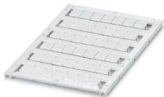
Marker for terminal blocks, can be ordered: by sheet, white, labeled according to customer specifications, mounting type: snap into tall marker groove, for terminal block width: 8.2 mm, lettering field size: 7.6 x 10.5 mm, Number of individual labels: 42
