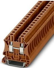
Feed-through terminal block, nom. voltage: 1000 V, nominal current: 41 A, number of connections: 2, connection method: Screw connection, Rated cross section: 6 mm<sup>2</sup>, cross section: 0.2 mm<sup>2</sup> - 10 mm<sup>2</sup>, mounting type: NS 35/7,5, NS 35/15, color: brown
