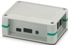
Complete housing for printed-circuit boards. Includes housing half shells, side panels with openings for all relevant connections, adhesive pads for affixing the Raspberry Pi model B2 and B3 computers, screws for housing and PCB attachment; light gray housing with turquoise-blue corner inlays
