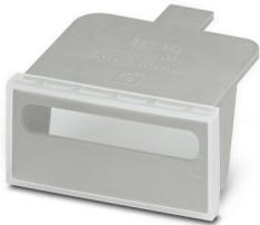
Marker carriers, for the identification of terminal block groups, for E/UK end bracket or E/U end bracket, with 40 x 17 mm perforated insert strip, gray, unlabeled, perforated, mounting type: snapped, lettering field size: 40 x 17 mm
