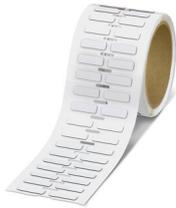
Label, Roll, white, unlabeled, can be labeled with: THERMOMARK E.300 (D)/600 (D), THERMOMARK ROLL 2.0, THERMOMARK ROLL, THERMOMARK ROLL X1, THERMOMARK ROLLMASTER 300/600, THERMOMARK X1.2, mounting type: adhesive, lettering field size: 27 x 8 mm, Number of individual labels: 500
