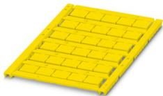
Marker for terminal blocks, Sheet, yellow, unlabeled, can be labeled with: TOPMARK NEO, TOPMARK LASER, BLUEMARK ID COLOR, BLUEMARK ID, BLUEMARK CLED, THERMOMARK PRIME, THERMOMARK CARD 2.0, THERMOMARK CARD, mounting type: snapped, for terminal block width: 12 mm, lettering field size: 10.8 x 9.6 mm, Number of individual labels: 30
