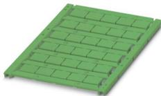
Marker for terminal blocks, Sheet, green, unlabeled, can be labeled with: TOPMARK NEO, TOPMARK LASER, BLUEMARK ID COLOR, BLUEMARK ID, BLUEMARK CLED, THERMOMARK PRIME, THERMOMARK CARD 2.0, THERMOMARK CARD, mounting type: snapped, for terminal block width: 12 mm, lettering field size: 10.8 x 9.6 mm, Number of individual labels: 30
