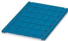
Marker for terminal blocks, Sheet, blue, unlabeled, can be labeled with: TOPMARK NEO, TOPMARK LASER, BLUEMARK ID COLOR, BLUEMARK ID, BLUEMARK CLED, THERMOMARK PRIME, THERMOMARK CARD 2.0, THERMOMARK CARD, mounting type: snapped, for terminal block width: 12 mm, lettering field size: 10.8 x 9.6 mm, Number of individual labels: 30
