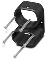
CHARX connect standard, Repair kit, Accessories, with replaceable mating face frame, with 5x M4X45 rounded head screws with Torx security drive, for replacement of the mating face frame of vehicle charging connectors, CCS type 2, IEC 62196-3, housing: black, The vehicle connector housing does not have to be opened in order to replace the mating face frame.
