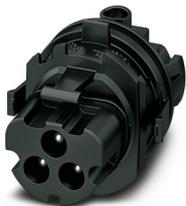
Contact insert, Range of articles: PRC 35, Contact carrier, housing material: PPE, color: black, number of positions: 3, min. conductor cross section: 1.5 mm<sup>2</sup>, max. conductor cross section: 6 mm<sup>2</sup>, rated voltage: 690 V AC, rated current: 35 A, Connection method: Screw connection, Contact connection type: Pin. Contact insert without connector housing. Please order the appropriate connector housings according to the accessories list.
