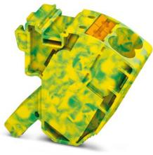
Pick-off terminal, nom. voltage: 1500 V, nominal current: 57 A, number of connections: 2, connection method: Push-in connection, 1 level, Rated cross section: 10 mm<sup>2</sup>, cross section: 0.5 mm<sup>2</sup> - 16 mm<sup>2</sup>, mounting type: on base element, color: green/yellow
