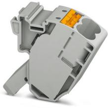
Pick-off terminal, nom. voltage: 1500 V, nominal current: 57 A, number of connections: 2, connection method: Push-in connection, 1 level, Rated cross section: 10 mm<sup>2</sup>, cross section: 0.5 mm<sup>2</sup> - 16 mm<sup>2</sup>, mounting type: on base element, color: gray
