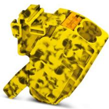
Pick-off terminal, nom. voltage: 1500 V, nominal current: 57 A, number of connections: 2, connection method: Push-in connection, 1 level, Rated cross section: 10 mm<sup>2</sup>, cross section: 0.5 mm<sup>2</sup> - 16 mm<sup>2</sup>, mounting type: on base element, color: black/yellow
