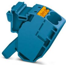
Pick-off terminal, nom. voltage: 1500 V, nominal current: 57 A, number of connections: 2, connection method: Push-in connection, 1 level, Rated cross section: 10 mm<sup>2</sup>, cross section: 0.5 mm<sup>2</sup> - 16 mm<sup>2</sup>, mounting type: on base element, color: blue
