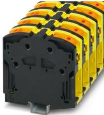
High-current terminal block, nom. voltage: 1000 V, nominal current: 309 A, number of connections: 2, number of positions: 1, connection method: PowerTurn connection, 1 level, cross section: 95 mm<sup>2</sup> - 185 mm<sup>2</sup>, mounting type: NS 35/15, color: black/yellow
