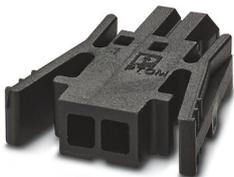
PCB connector, nominal cross section: 0.75 mm<sup>2</sup>, color: black, nominal current: 6 A, rated voltage (III/2): 160 V, contact surface: Tin, contact connection type: Socket, number of rows: 1, number of positions: 4, product range: PTCM 0,5/...-PL, pitch: 2.5 mm, connection method: Crimp connection, conductor/PCB connection direction: 0 °, plug-in system: COMBICON PTSM, locking: Snap-in locking, mounting: Self-locking flange, type of packaging: packed in cardboard
