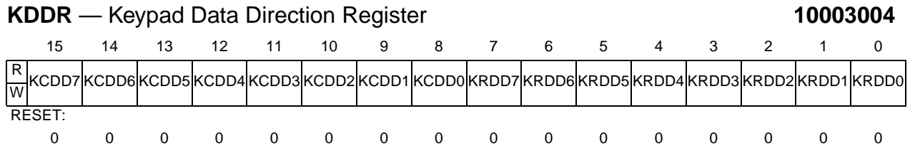
Figure 14-4 Keypad Data Direction Register
