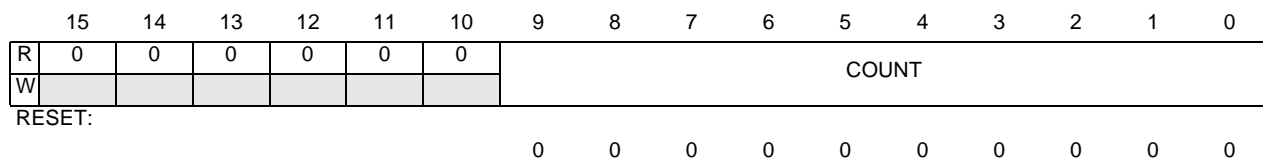
Figure 15-7 PWM Count Registers
