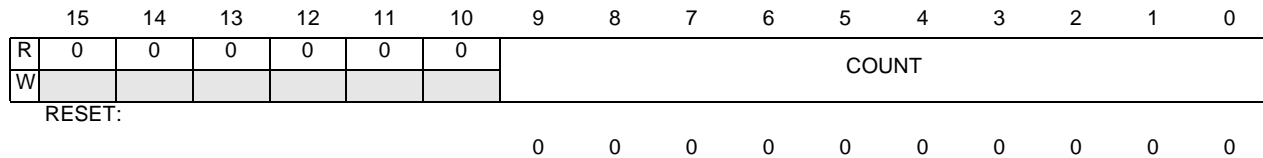
Figure C-27 PWM Count Registers
