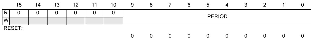
Figure 15-5 PWM Period Registers
