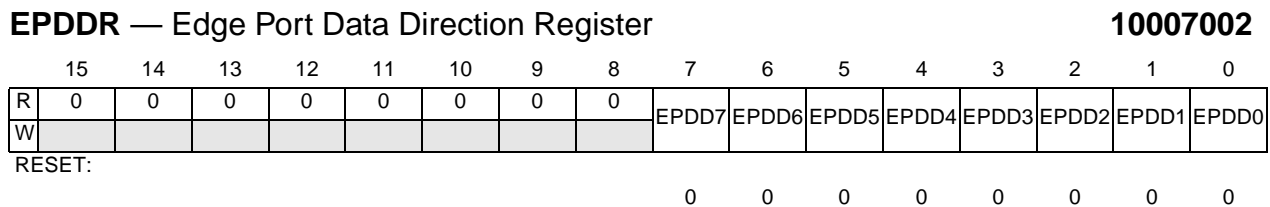
Figure 13-3 Edge Port Data Direction Register
