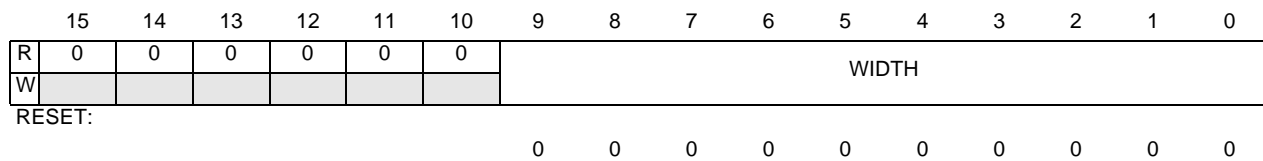
Figure 15-6 PWM Width Registers
