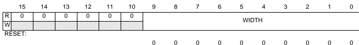
Figure C-26 PWM Width Registers
