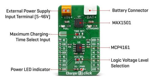
The MAX1501 IC is designed with reliability in mind: the IC prevents draining the battery below the critical level, protects it from overheating (if thermistor is used), offers prequel charging (for deeply depleted batteries), features an overvoltage protection, charging status monitoring and so on. The Click board™ itself is equipped with a set of indicators used to monitor both charging process and power distribution.
