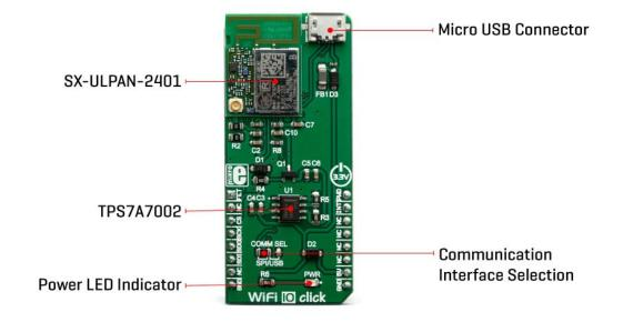
The ULPAN-SB-2401 module supports IPv4, TCP, and UDP transfer protocols, and complies with the IEEE802.11a/b/g/n wireless networking standards, at 2.4GHz. It supports data rates from 1 to 54 Mbps for 802.11b/g, and MCS from 0 to 7, for 802.11n. The SX-UPLAN-2401 module also provides support for WPS, WPA, and WPA2 security protocols, allowing a secure connection.
