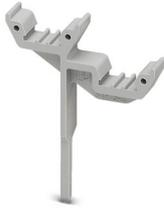
Marker carriers, snaps into the PT 1,5/S-3L Push-in three-level terminal block, can be marked with UCT-TM 3,5, UCT-TMF 3,5, ZB 3,5, or ZBF 3,5, gray, unlabeled, mounting type: plug in, lettering field size: 3.5 x 10.5 mm
