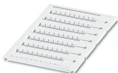
Marker for terminal blocks, Sheet, white, unlabeled, can be labeled with: BLUEMARK ID COLOR, BLUEMARK ID, BLUEMARK CLED, PLOTMARK, CMS-P1-PLOTTER, mounting type: snapped, for terminal block width: 5.2 mm, lettering field size: 5 x 7 mm, Number of individual labels: 80
