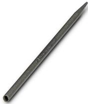
Threading pin, helps thread PMH onto the conductor; insert conductor into pin opening and slide collar on. For external conductor cross section: 2.0 - 2.5 mm
