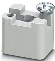
Support bracket made from insulation material, with retaining screw, can be used with either 3 x 10 mm or 6 x 6 mm busbar, color: gray
