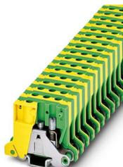
Ground terminal, When aligned with a feed-through terminal block of the same shape, a partition plate must be used for insulation voltages > 250 V, number of connections: 2, connection method: Screw connection, 1 level, cross section: 0.2 mm<sup>2</sup> - 4 mm<sup>2</sup>, mounting: PE foot with mounting screw, M3, mounting type: NS 15, color: green-yellow
