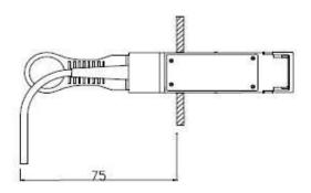
Clearance 75mm Is Required. Cable Type: Low Smoke Zero Halogen
