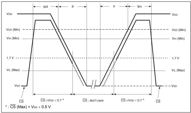
In case relative short  $V_{DD}$  pulse whose peak level is beyond 1.7 is applied, please set  $V_{DD}$  falling time, tf, longer than 0.4ms/V. (When  $V_{DD}$  rises beyond 1.7V, and falls just after, if this term is very short the device may loose its function.).
