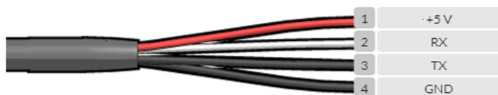
Communication cable pinout
