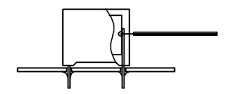
Temperature monitored inside the capacitor.
