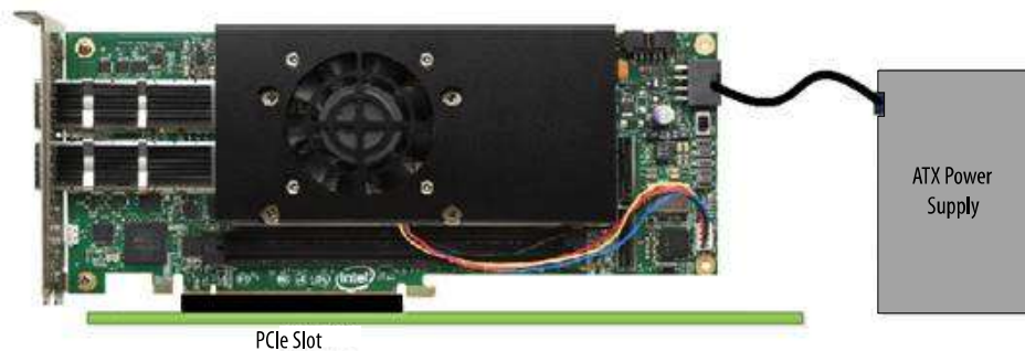
Figure 37. Powering Board Using Standard PCIe-Compliant System
