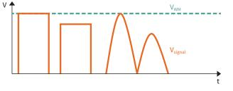
Fig. 6 V<sub>WM</sub> equal or higher than V<sub>signal</sub>
