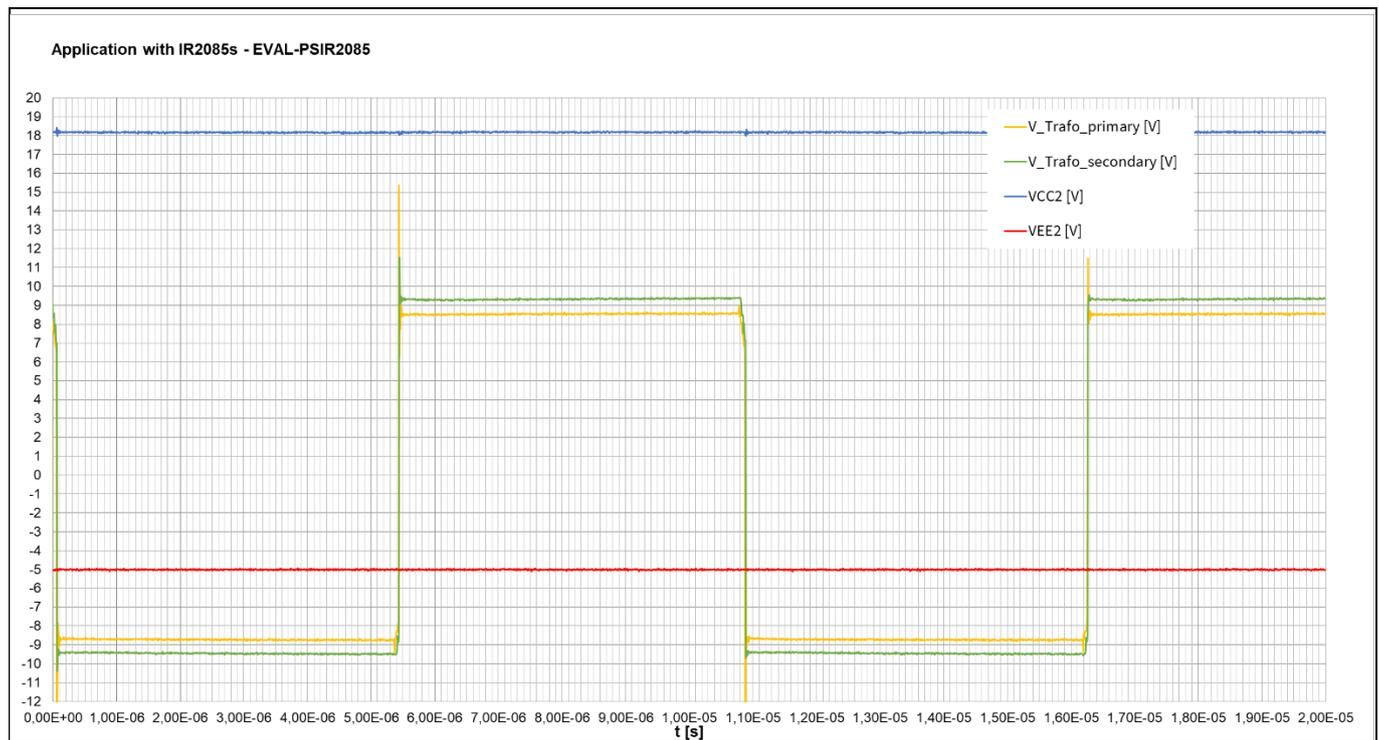
**Figure 11 Normal operation of the power supply board**
