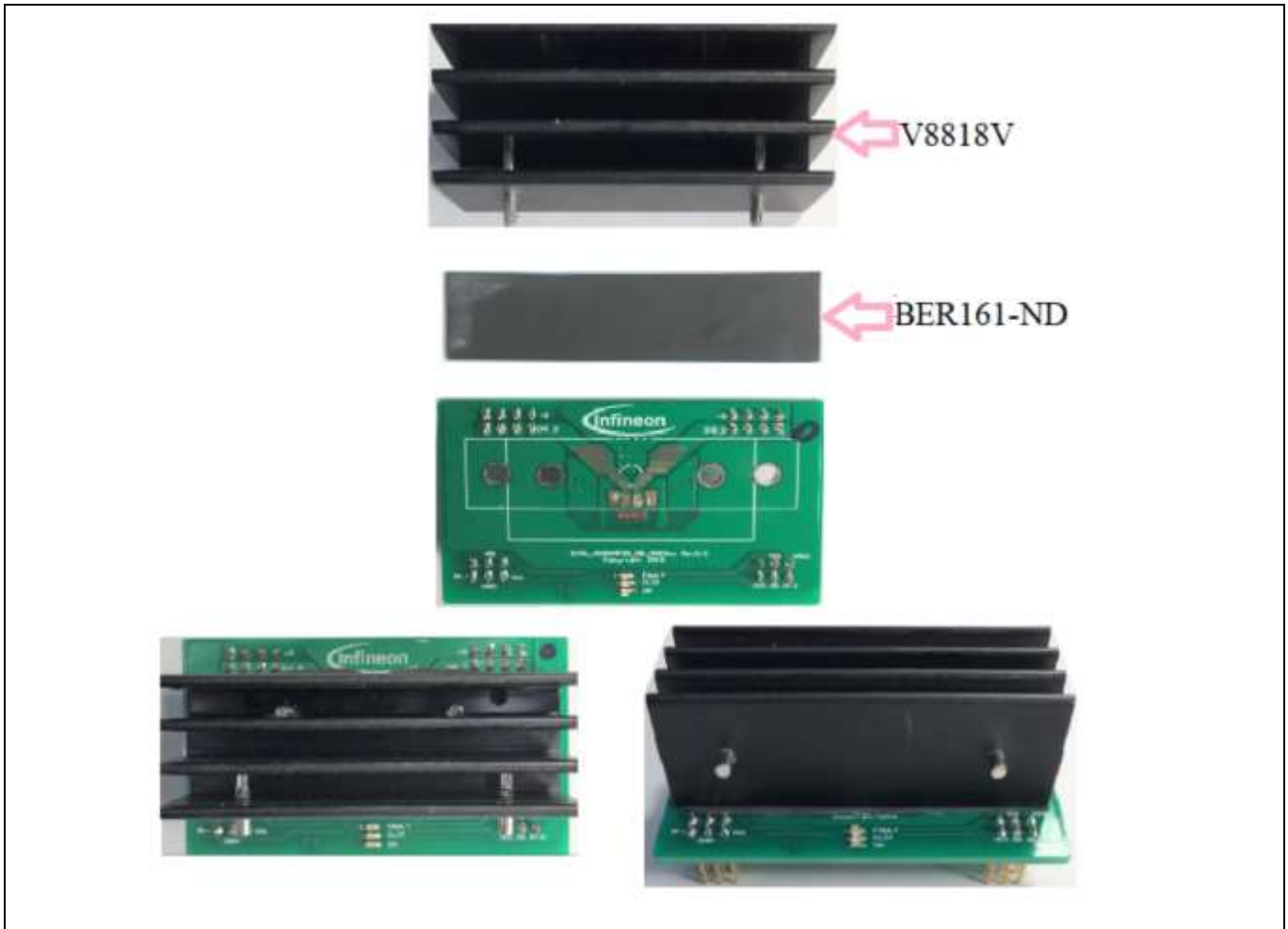
Figure 15 Heatsink installation
