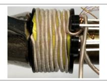
Figure 17 Secondary part of the primary winding
