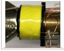
Figure 18 Insulation layer 4
