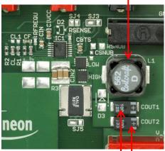
Output Filter Capacitors C<sub>OUT</sub>
