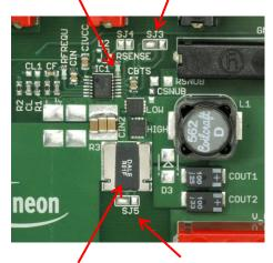
Shunt Resistor R<sub>SHUNT</sub>
