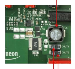
Output Filter Capacitor C<sub>OUT</sub>
