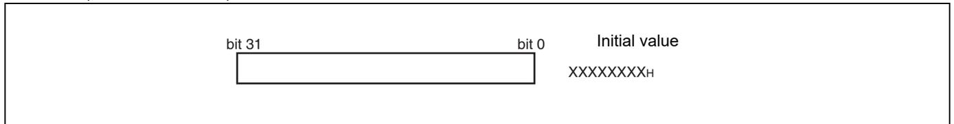
The user stack pointer, when the S flag is "1", this register functions as the R15 register.
