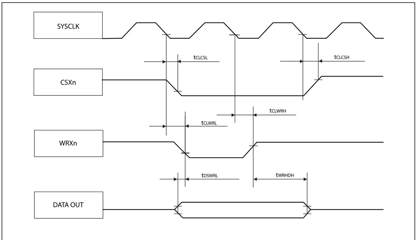
Asynchronous Write Access - Byte Control Type
