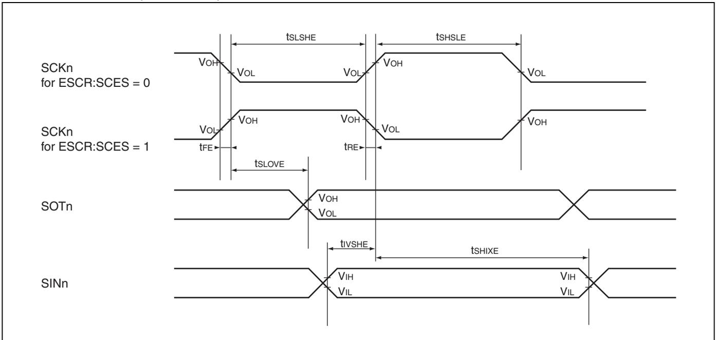
**16.7.4 I<sup>2</sup>C AC Timings at V<sub>DD5</sub> = 3.0 to 5.5 V**
