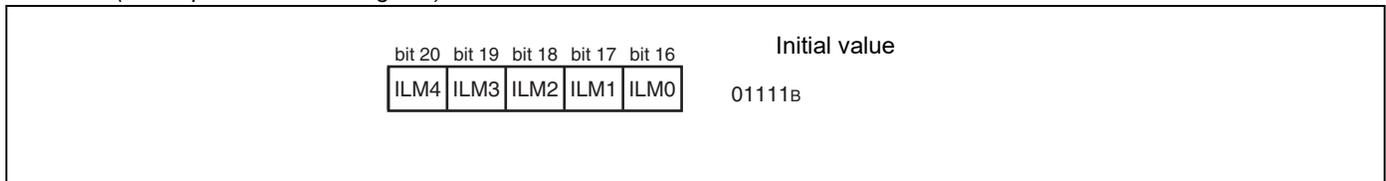
This register stores interrupt level mask values, and the values stored in ILM4 to ILM0 are used for level masking.
