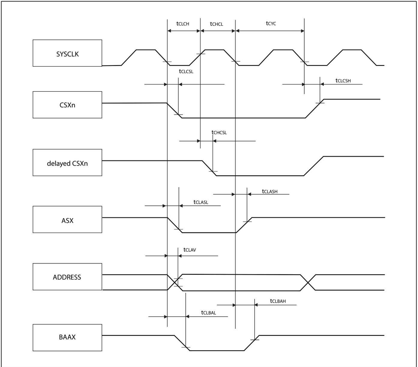
*Synchronous/Asynchronous Read Access with External MCLKI Input*
