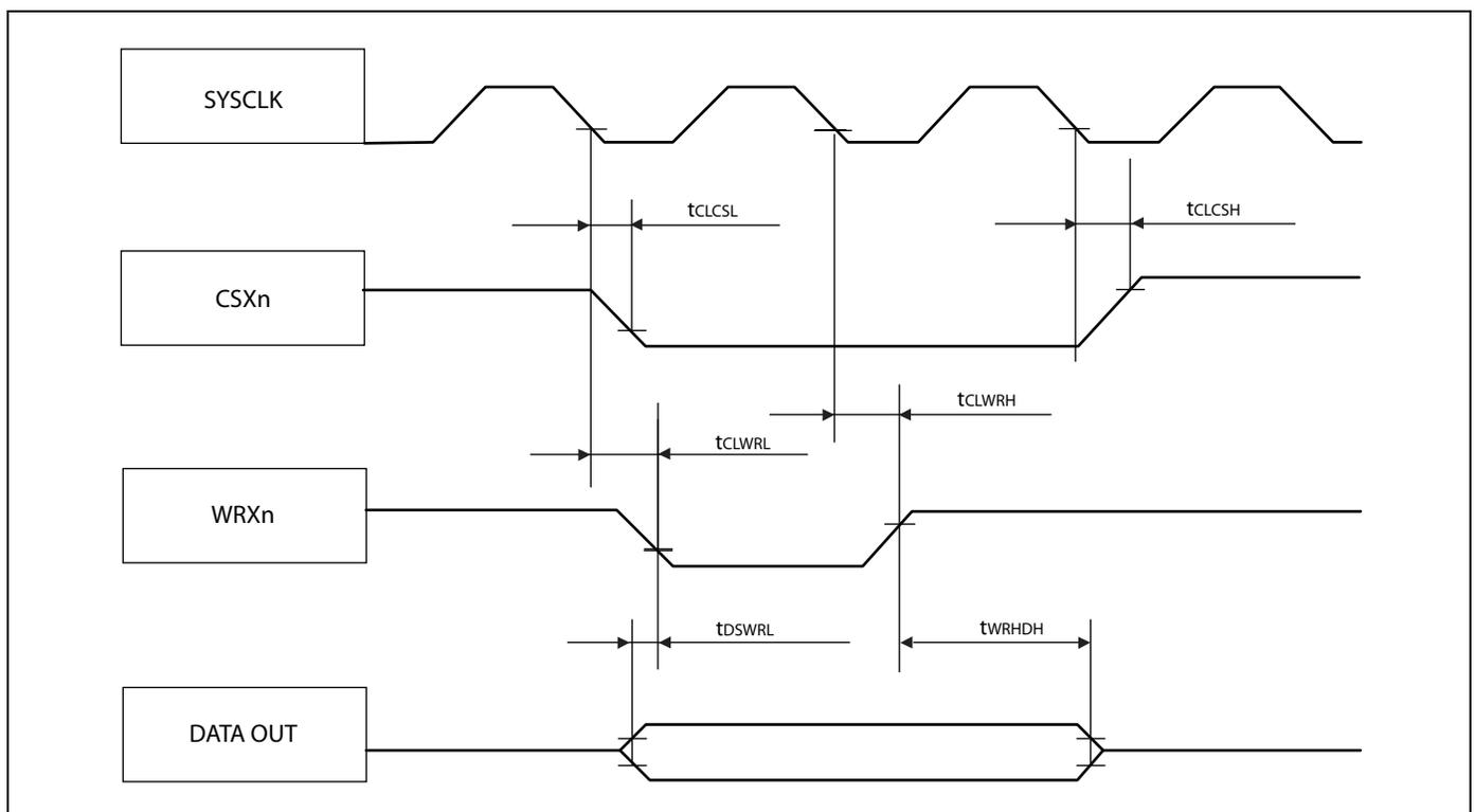
Asynchronous Write Access - Byte Control Type
