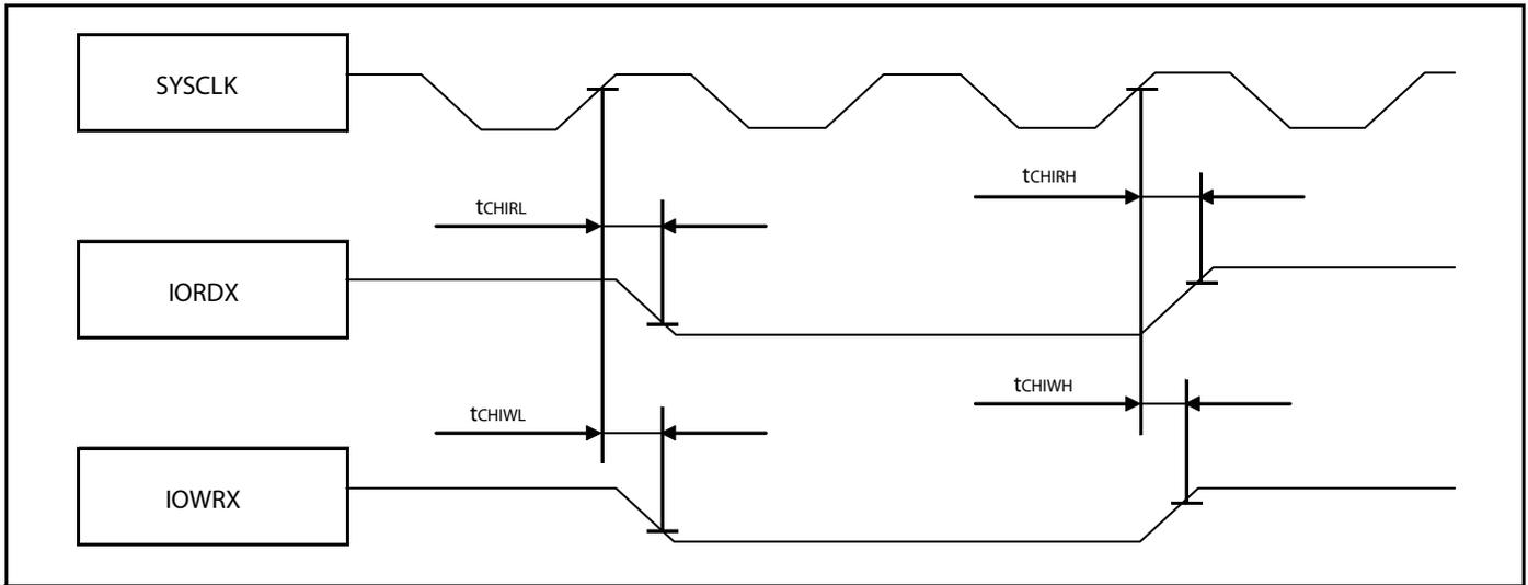
**16.7.8 External Bus AC Timings at  $V_{DD35} = 3.0$  to  $4.5$  V**
