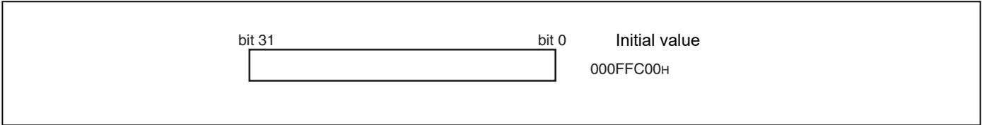
The table base register stores the starting address of the vector table used in EIT processing.
