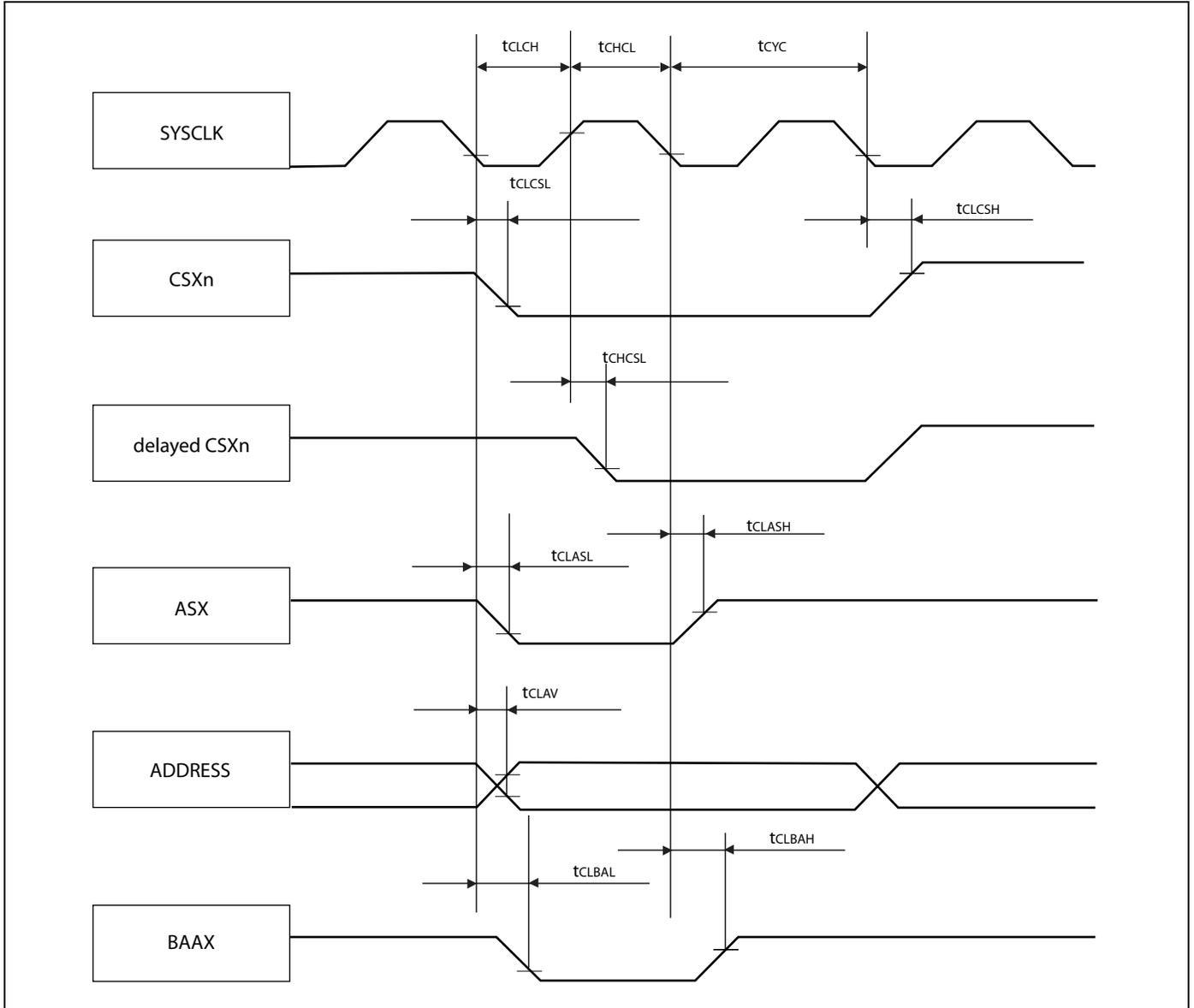
*Synchronous/Asynchronous Read Access with External MCLKI Input*
