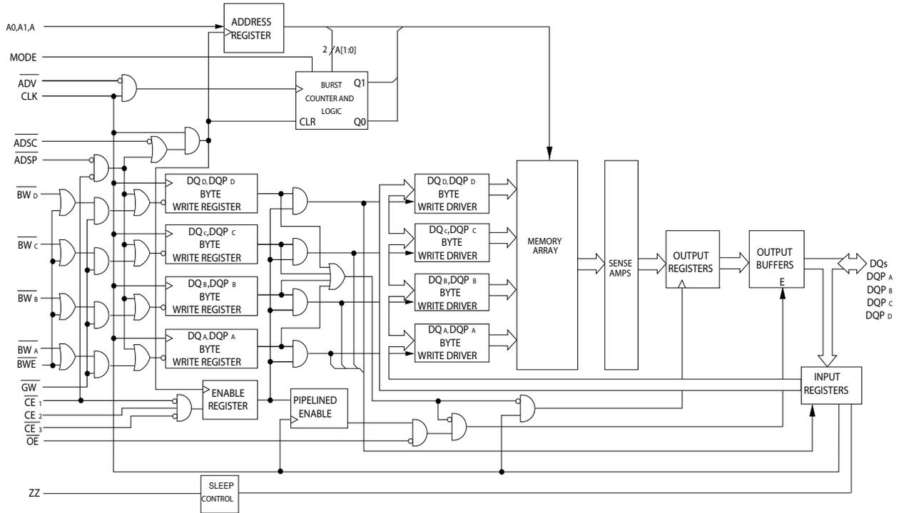
**Logic Block Diagram – CY7C1387KV33**
