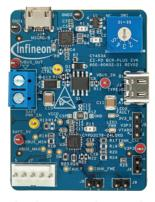
The CY4534 EZ-PD™ barrel connector replacement-plus (BCR-PLUS) EVK is an evaluation platform for customers who want to replace an existing barrel/power input connector with a USB-C connector using the CYPD3176 device. Implementing this solution in an end-product allows the system to be powered by any USB-PD compliant power adapter or any USB power adapter that supports legacy charging standards.
