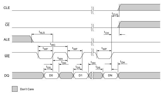
Figure 5. Data Input Cycle
