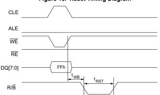
Figure 16. Reset Timing Diagram
