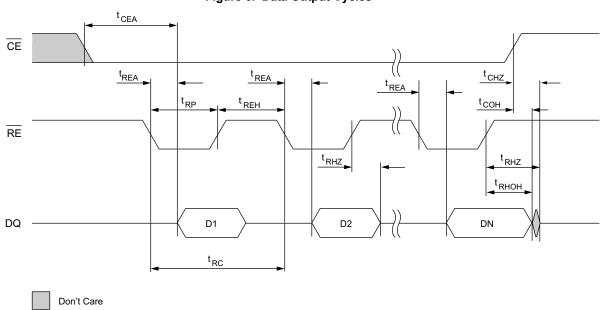
Figure 6. Data Output Cycles
