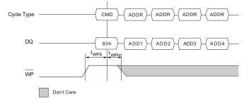
Figure 22. Write Protect Enable Timing
