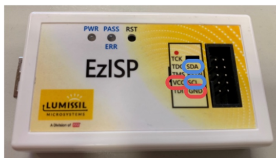
Figure 47: Pin configuration on EzISP board
