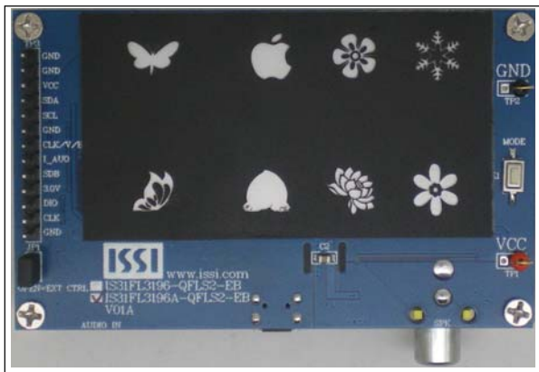
Figure 1: Photo of IS31FL3196A Evaluation Board
