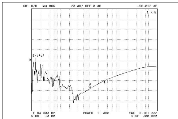
FIGURE 2-14: PSRR2-VPP (VPP = 225V + 1V AC).
