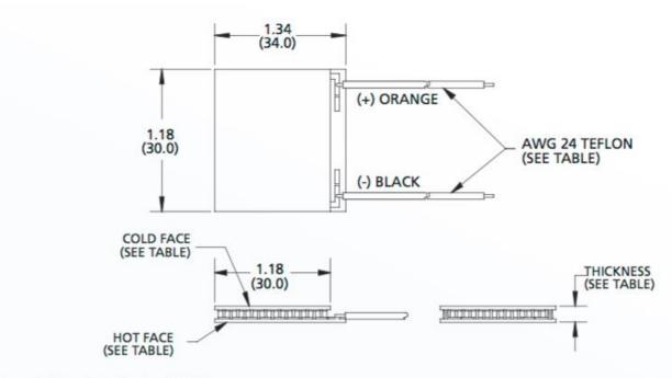
Ceramic Material: Alumina (Al<sub>2</sub>O<sub>3</sub>) Solder Construction: 271°C, Proprietary
