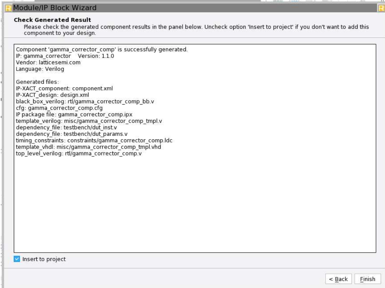
Figure 3.3. Check Generating Result
