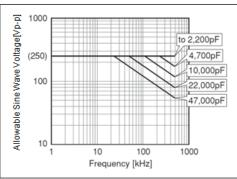
Chip(LxW): 3.2x1.6mm/3.2x2.5mm/ 4.5x3.2mm/5.7x5.0mm U2J(7U) Char. Rated Voltage:DC500V
