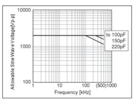
Chip(LxW): 4.5x2.0m U2J(7U) Char. Rated Voltage:DC3.15kV
