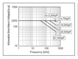
Chip(LxW): 2.0x1.25mm/3.2x1.6mm U2J(7U) Char. Rated Voltage:DC250V
